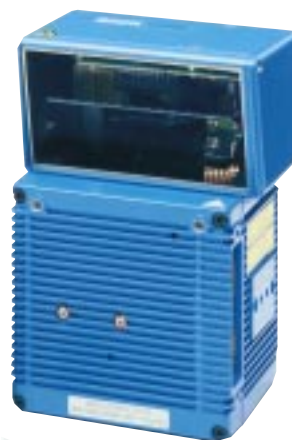
Line scanner with oscillating mirror
