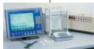
Testplace module with weighing station, tablet tester and dimension measurement
