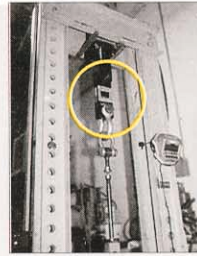
Tension testing and calibration
